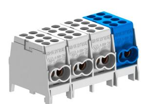
4-pin main terminal block,  $2 \times 16 \text{ mm}^2 + 2 \times 25 \text{ mm}^2$  conductor connection cross-sections per pin. With 2 screws per terminal for secure contact pressure. High-resistance quick-action fastening made of galvanised sheet steel for simple mounting on support rails.
