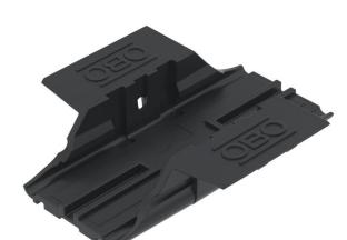
Adapter for TP 45 support profile, for mounting on UniBase universal stand. Toolless mounting through snapping. With side holes for optional screwing. Toolless mounting and dismantling of the support profile possible. With non-slip support surface.
