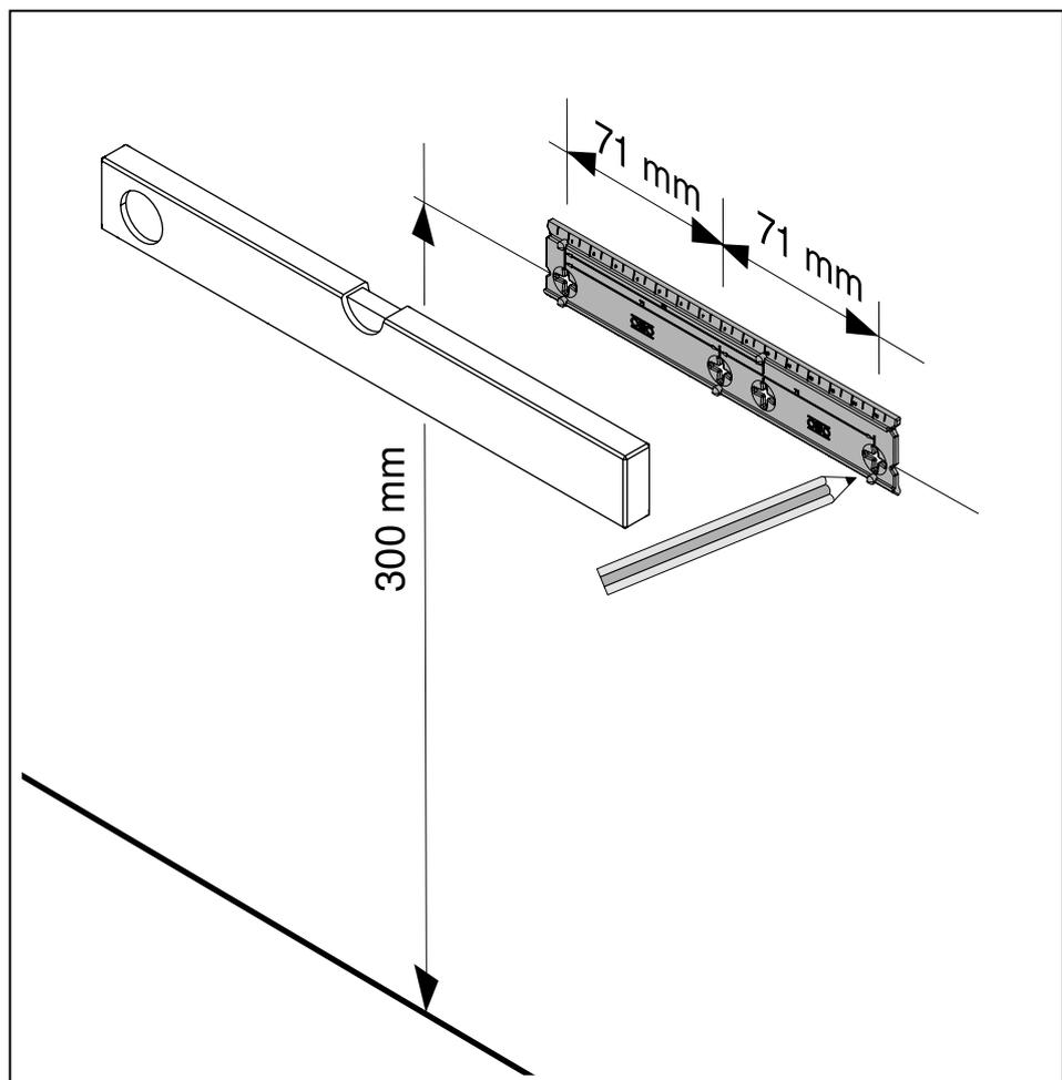
Fig. 5: Drawing on the drill hole
