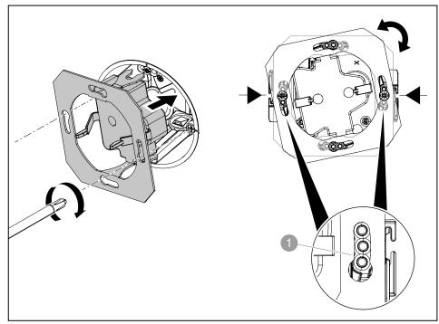
Fig. 20: Inserting a device
