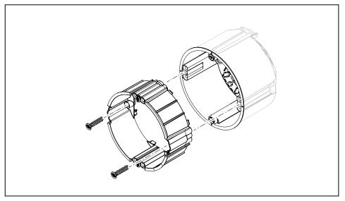
Fig. 23: Mounting a compensation ring
