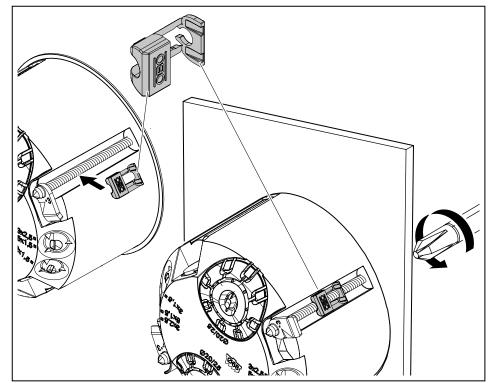
Fig. 16: Applying the fastening element
