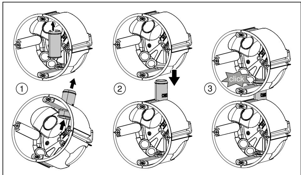
Fig. 15: Insert the connector
