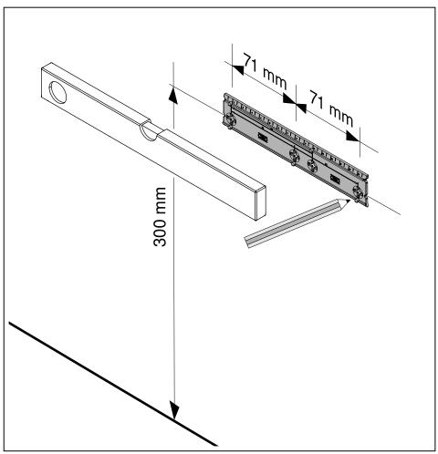
Fig. 5: Drawing on the drill hole
