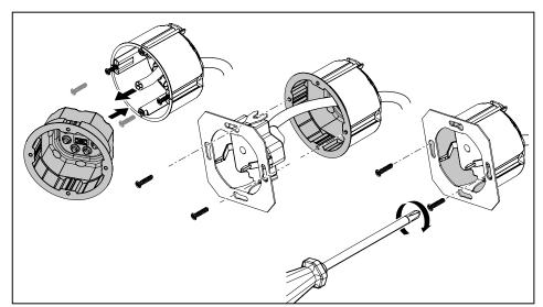
Fig. 22: Inserting a sealing insert with a device
