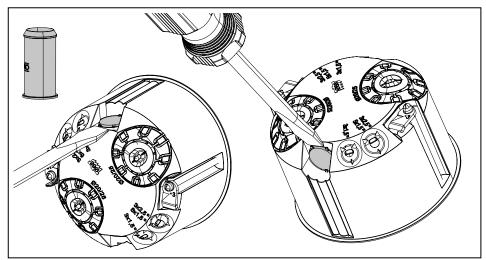
Fig. 12: Creating an opening for the connector on the standard box
