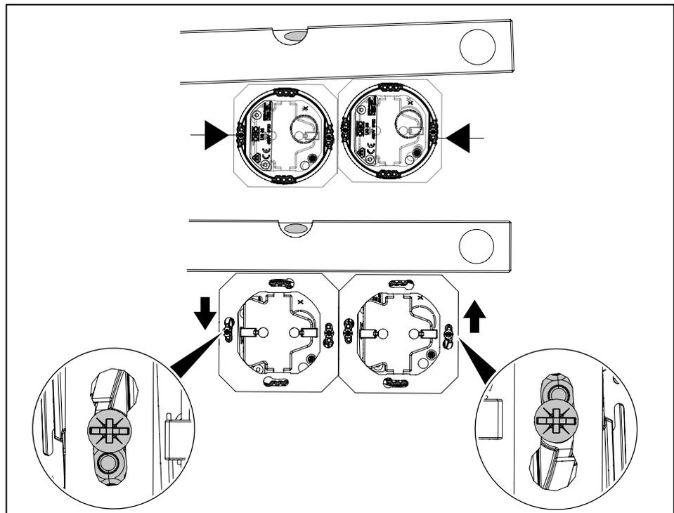
**Fig. 21:** Aligning multiple devices
