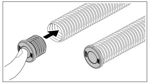
Fig. 25: Inserting the sealing plug
