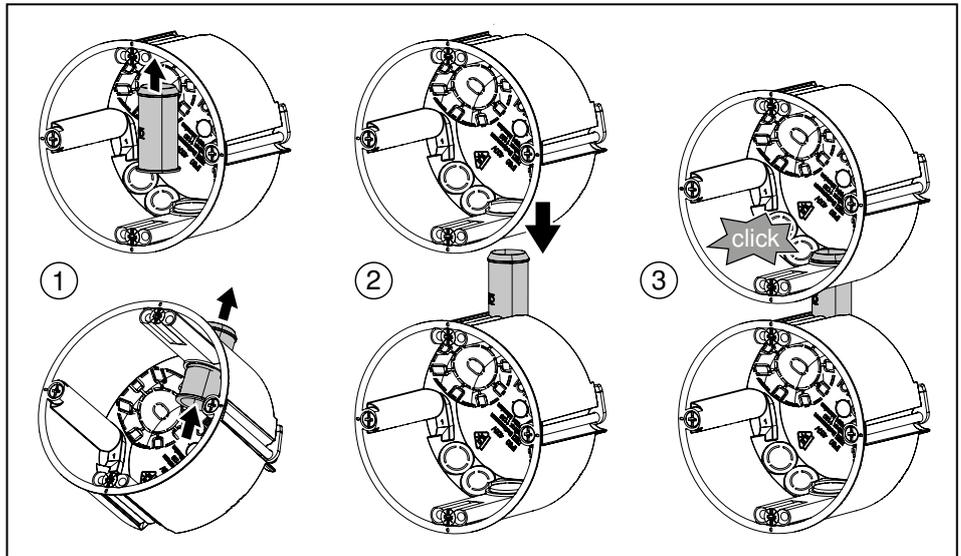
Fig. 13: Inserting and connecting connectors
