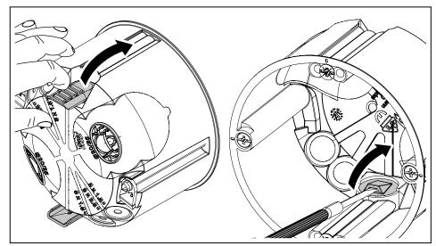
Fig. 14: Creating an opening for the connectors on an airtight box
