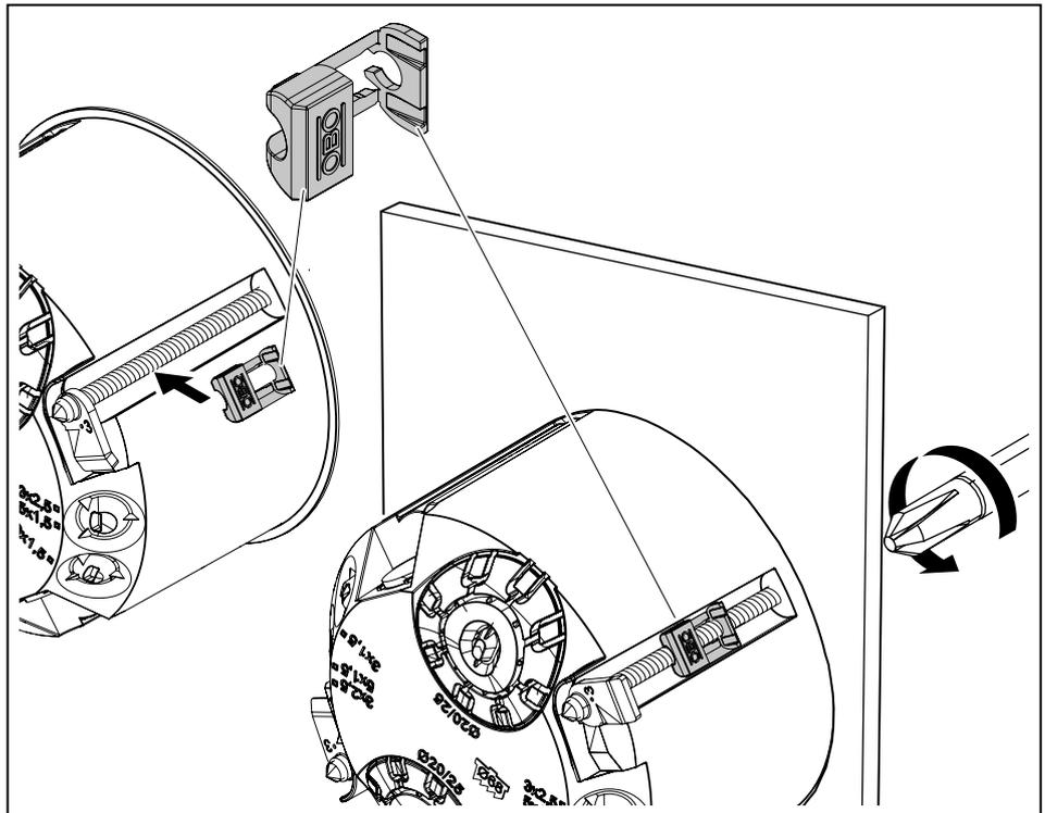
Fig. 16: Applying the fastening element
