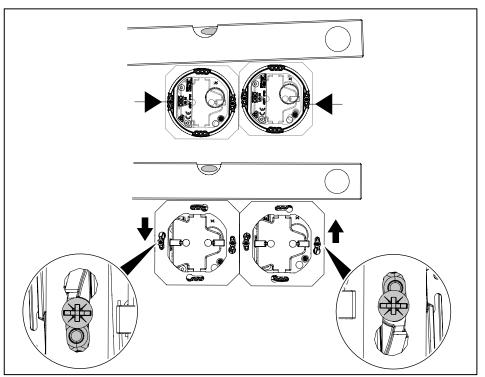
Fig. 21: Aligning multiple devices
