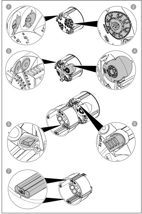
Fig. 3: Details, cavity wall boxes
