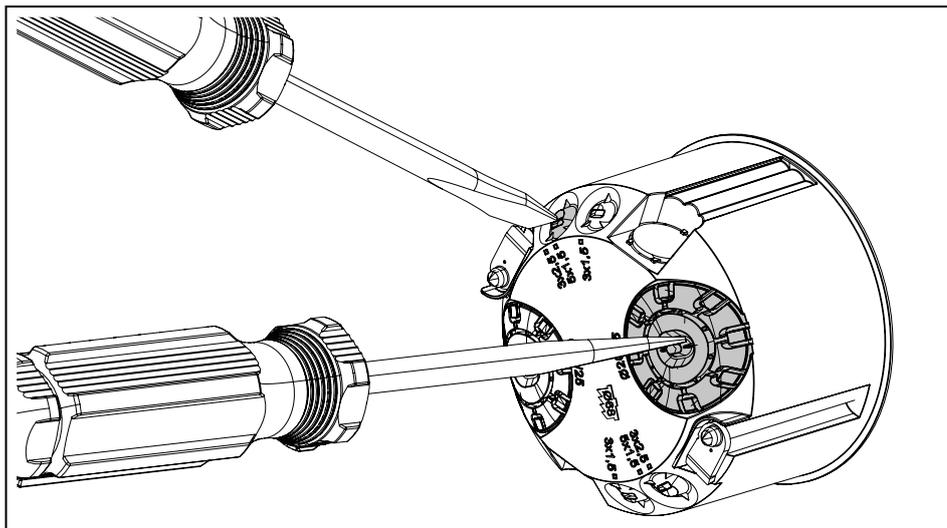
**Fig. 7:** Breaking out the break-out openings
