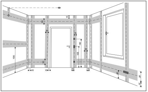
Fig. 4: Installation zones, dimensions in cm
