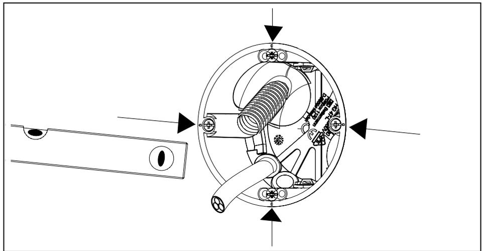
**Fig. 10:** Aligning the cavity wall box
