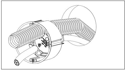
Fig. 8: Inserting the cable and corrugated pipe into the cavity wall box
