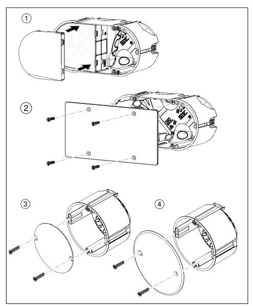
Fig. 27: Mounting the cover
