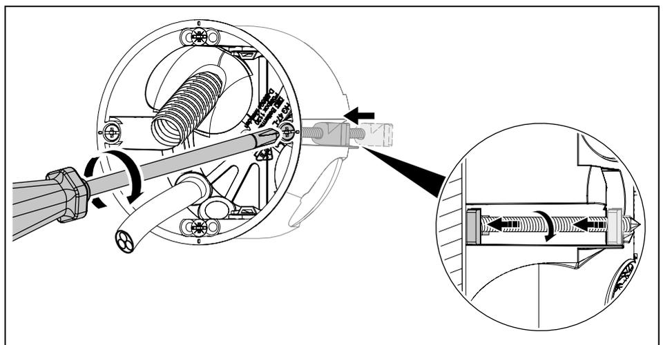
**Fig. 11:** Fixing the cavity wall box
