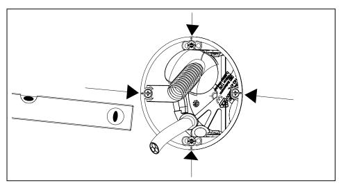
Fig. 10: Aligning the cavity wall box
