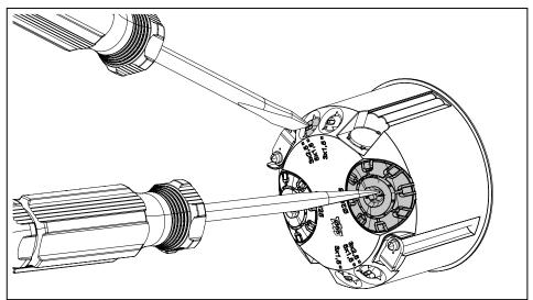
Fig. 7: Breaking out the break-out openings
