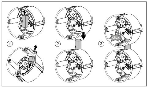
Fig. 13: Inserting and connecting connectors
