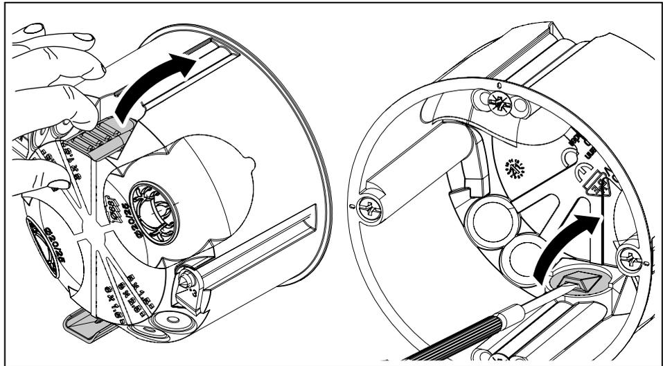
Fig. 14: Creating an opening for the connectors on an airtight box
