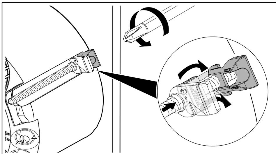
**Fig. 18:** Clamping the fastening element
