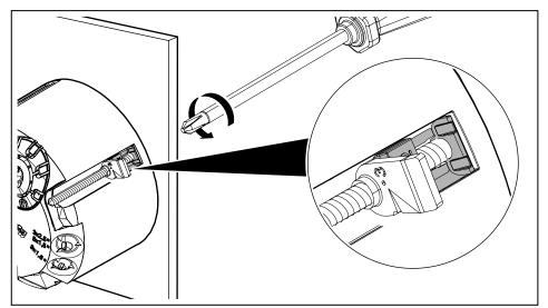
Fig. 17: Tightening the clamping lug
