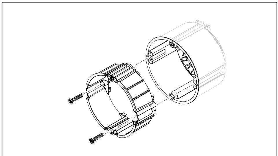
**Fig. 23:** Mounting a compensation ring
