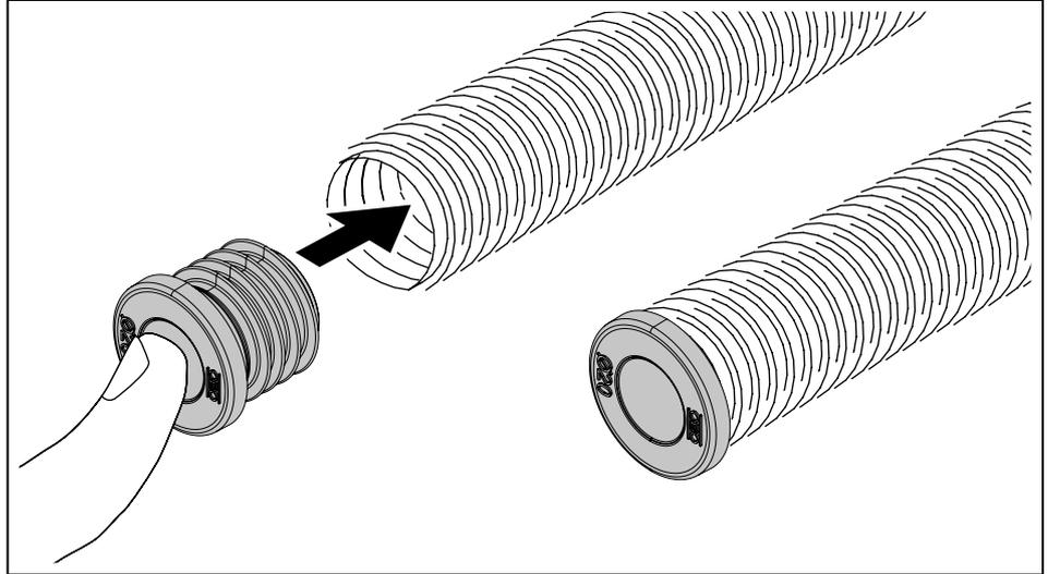
Fig. 25: Inserting the sealing plug
