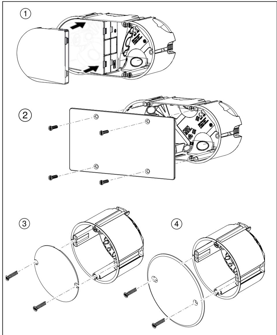
**Fig. 27:** Mounting the cover
