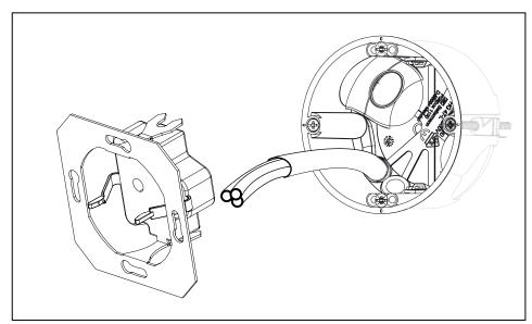
Fig. 19: Connect the device with cables
