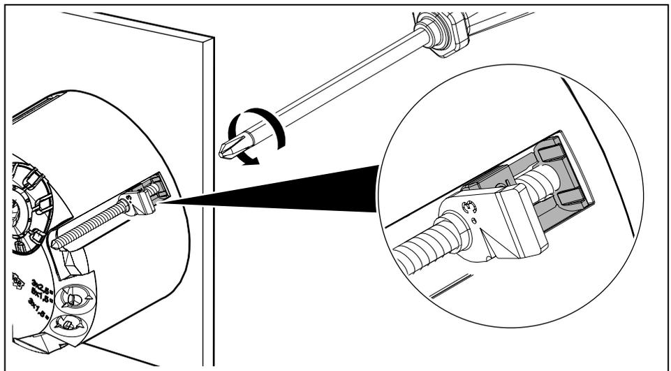
Fig. 17: Tightening the clamping lug
