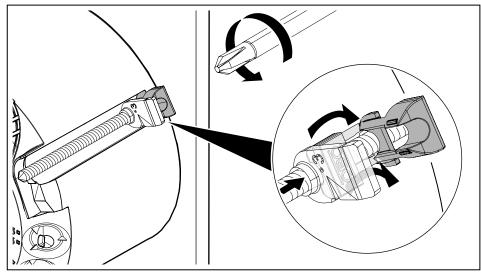
Fig. 18: Clamping the fastening element
