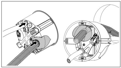
Fig. 9: Inserting the cable and corrugated pipe into the airtight cavity wall box
