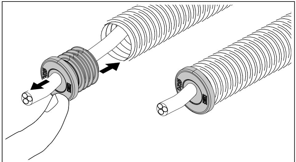
Fig. 26: Inserting sealing plug with cable
