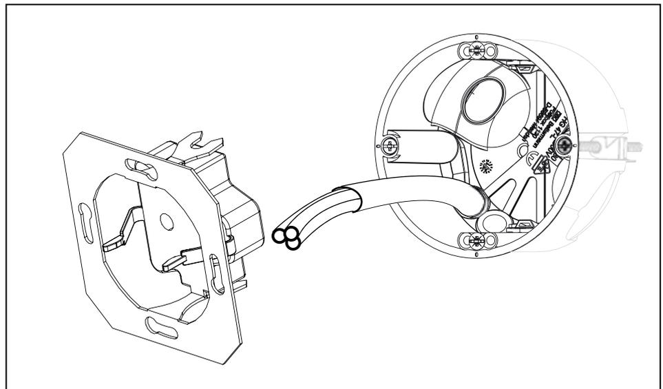
**Fig. 19:** Connect the device with cables
