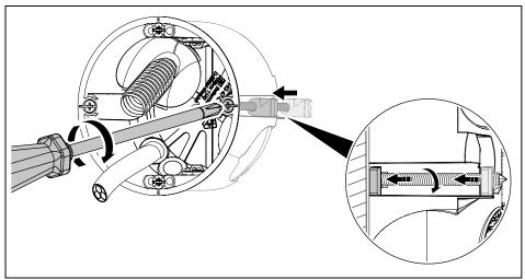
Fig. 11: Fixing the cavity wall box
