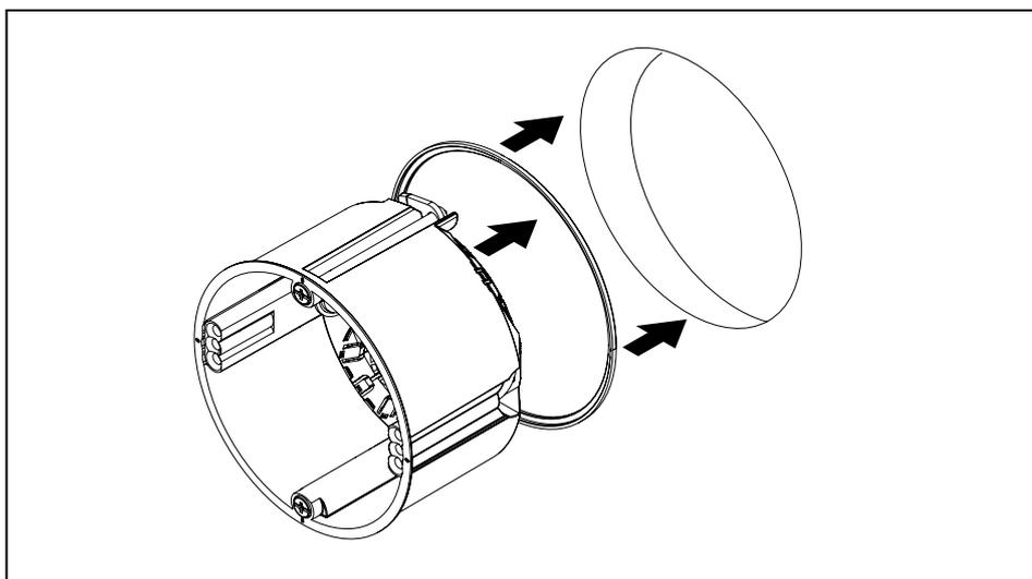
**Fig. 24:** Inserting the compensation ring
