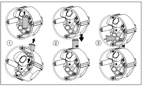
Fig. 15: Insert the connector
