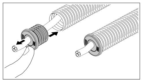
Fig. 26: Inserting sealing plug with cable
